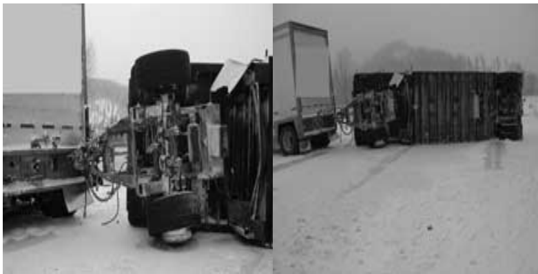
Photo 1. Dolly used to pull second trailer in tandem. (Photo courtesy of State Highway Patrol)
